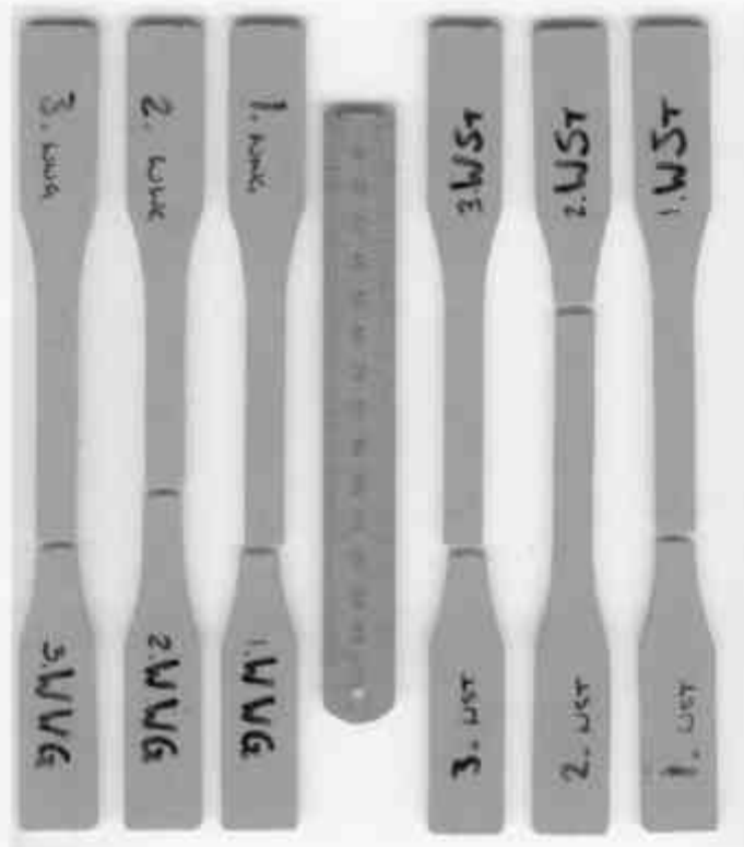
Figure 3. Dumb bell specimens after test
