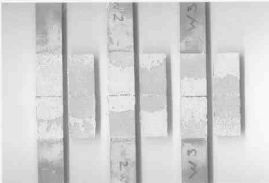
Figure 6. Double lap shear specimens after test (Winter Grade)
